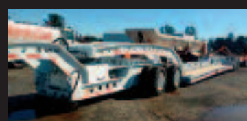
1995 COZAD BABY 9-AXLE 2+2+2 LOWBED, 9' wide x 26' deck, drop sides, power tower in jeep w/20 hp Honda, 4 pin settings. Following items are NEW: all wheel studs, all 11R22.5 tires, all drums, all brakes, all bearings, all slacks, all S-cams, all lights, all wiring, all air lines, all air valves, all apitong deck, all oil caps, all seals, all air bags, all paint + more.....$135,000
