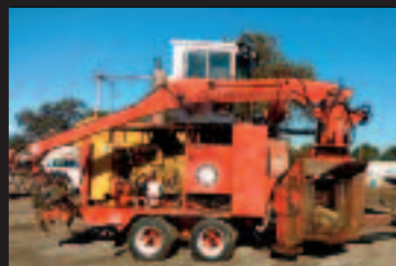
MORBARK 20 CHIPPER, new CAT C13 with 3,684 hours, 385 hp, Tier III, new tires, good brakes, lights.....$69,500
