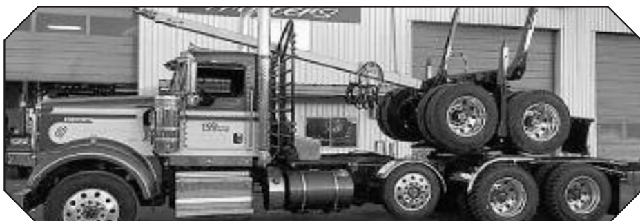
David Kehr , TILLAMOOK, OR, Brand New 2017 Whit-Log SEWC100 Long Logger with Matching Truck Equipment. Custom Steel Cab Rack, Double Tapered Stinger, Custom light bars, and Much More... Thanks David!!
