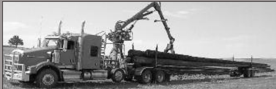
NEW SERCO 160PH POLE HANDLING PACKAGE IN STOCK, lifts up to 110' poles
