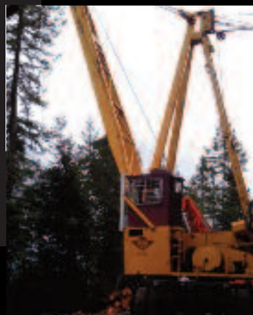
WASHINGTON 188 YARDER, Detroit 8V92T power, 4-axle carrier, standing skyline. This is a good, clean unit that was working as of 06/10/16. Consigned, call for location.....$250,000
