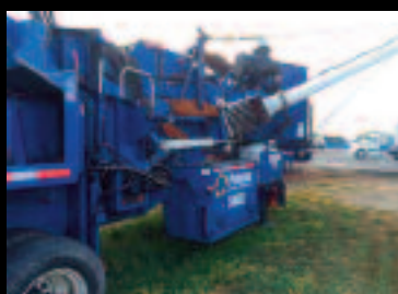
2010 PETERSON PACIFIC 5900EL CHIPPER, low hours, CAT power @ 765 hp, C18, remote, 4-pocket disc, P.T. Tech hyd clutch, 3/4" chip size, end load spout, 300 gal. water tank w/pump for fire suppression, IQAN screen, 2,400 hours, very good unit, consigned, west coast location.....$225,000
