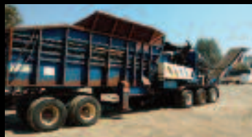
1996 PETERSON 4400B GRINDER, CAT 3412 @ 800 hp, 3 axles, all new tires, twin-disc clutch, dual horizontal rams for feed, heavy rotor, good last clean older unit, approx 87,000 lbs. w/o tractor.....$79,500
