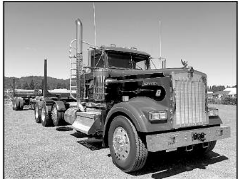
Log truck upfit with custom aluminum cab rack, scaler platforms, 12" Protech steps, Merritt decking, and custom paint of bunks and bolsters! Thanks John McNamara for your business!
