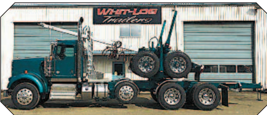
Russell Watkins Inc., PHILOMATH, OR , Brand New 2018 Whit-Log SEWC100 Long Loggers with Matching Truck Equipment. Custom Aluminum Cab Rack, Double Tapered Stinger, Double Drop in Chain Boxes, and Much More... Thanks Russell!!
