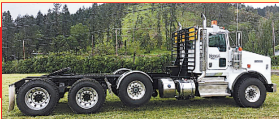
Nygaard Logging, WARRENTON, OR, (2) Brand New 2018 Whit-Log Lowboy Truck Equipment assemblies. Custom Steel Cab Rack, Complete Wet Kit, Custom Air/Electric/Hydraulic Station, and Much More... Thanks Matt!!
