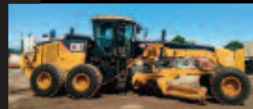
2008 CAT 14M VHP, 16' board, push block, rear ripper, good 20.5 tires, AC, Accugrade-ready, clean unit, Tier III, runs & shifts well, 8,155 hours.....$155,000
