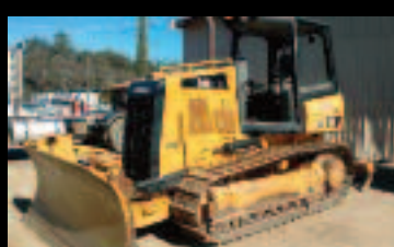
2015 CAT D4K2 XL 6-way dozer, rear ripper, open ROPS, wired, fair undercarriage, 2,087, just off job.....$79,500
